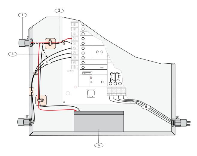
Figure 4.2: Non-PowerLimited Wiring
